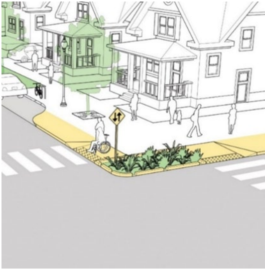
Figure 11-4: Bulb-Out Illustration (Source: National Association of City Transportation Officials (NACTO))
