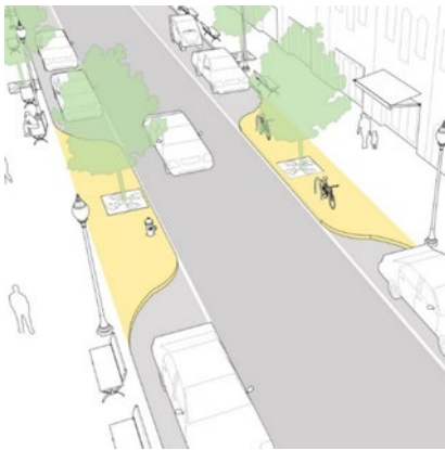
Figure 11-3: Pinchpoint Illustration (Source: National Association of City Transportation Officials (NACTO))
