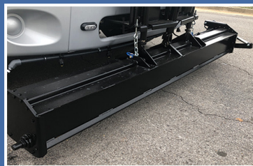
POWERFUL MAGNET TO COLLECT FERROUS MATERIAL
