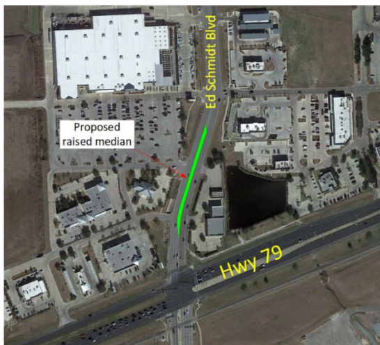
Figure 4. Recommended raised median
