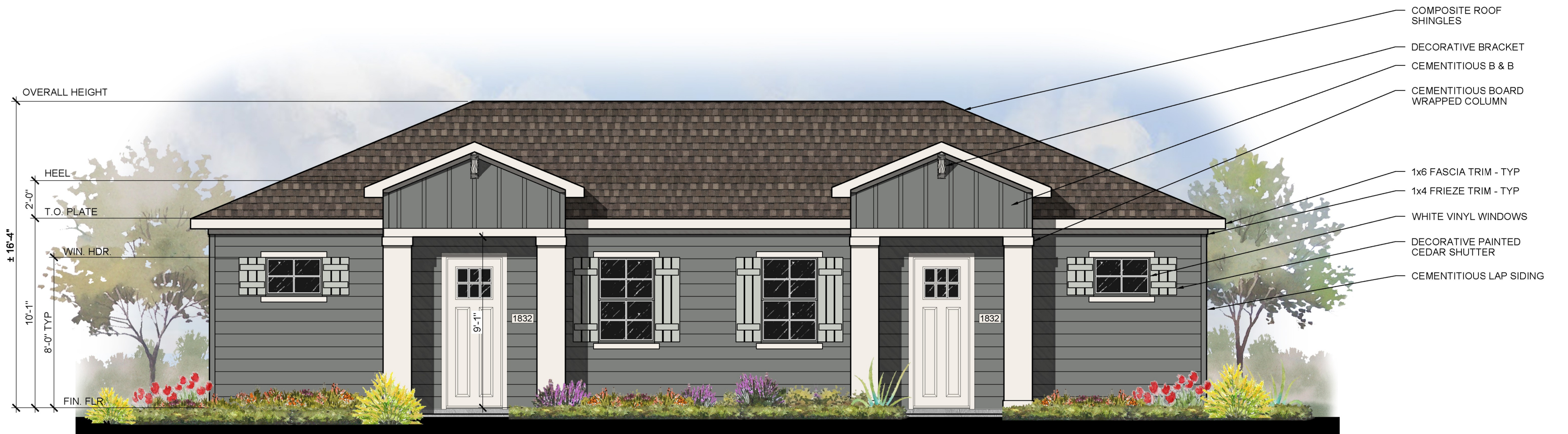
FRONT ELEVATION ELEVATION B - CALABASH 1/4" = 1'-0"
