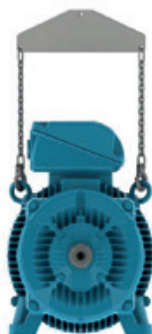
Figure 4.6 - Use of a spreader beam for lifting
