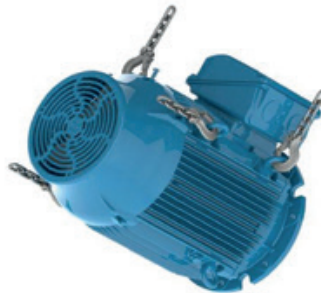
Figure 4.18 - Motor is being rotated to horizontal position
