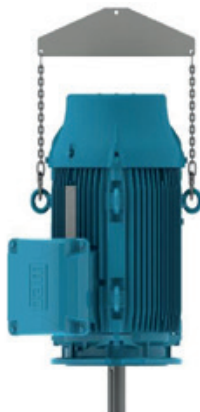
Figure 4.7 - Lifting of vertical mounted motors
