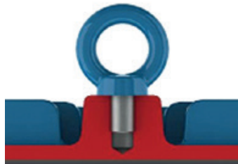
Figure 4.1 - Correct tightening of the eyebolt
