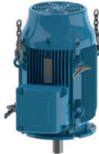
Figure 4.17 - Install the second pair of eyebolts
