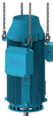
Figure 4.8 - Lifting of HGF and W50 motors.
