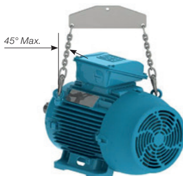
Figure 4.4 - Maximum resulting angle for motors with two or more lifting eyebolts
