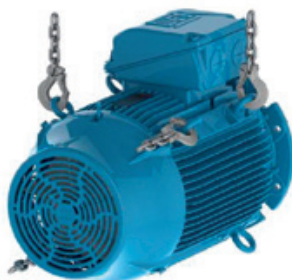
Figure 4.10 - Installation of the second pair of eyebolts
