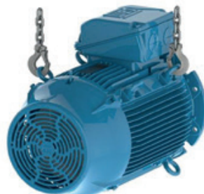
Figure 4.19 - Final result: motor placed in horizontal position
