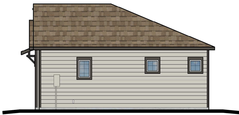
Right Elevation Elevation C 1/8" = 1'-0"
