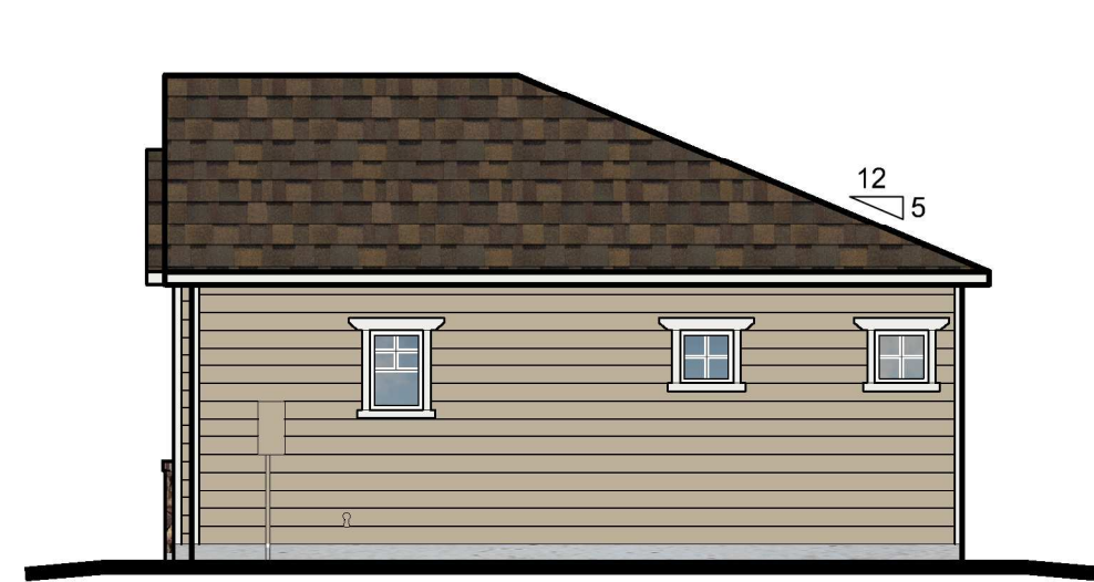
Right Elevation Elevation B 1/8" = 1'-0"
