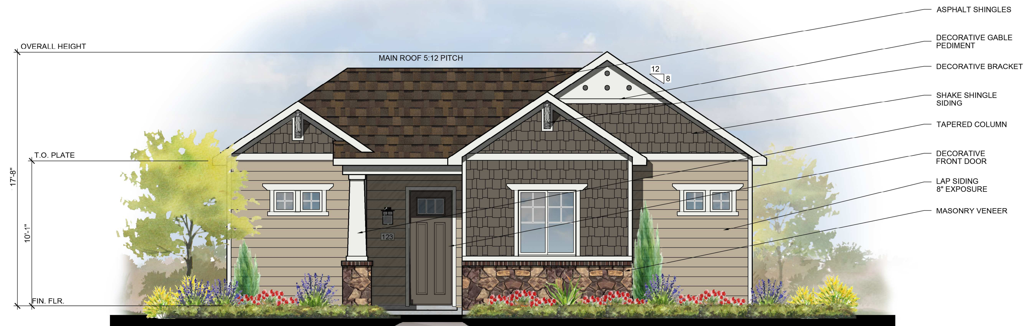
Front Elevation Elevation B 1/4" = 1'-0"
