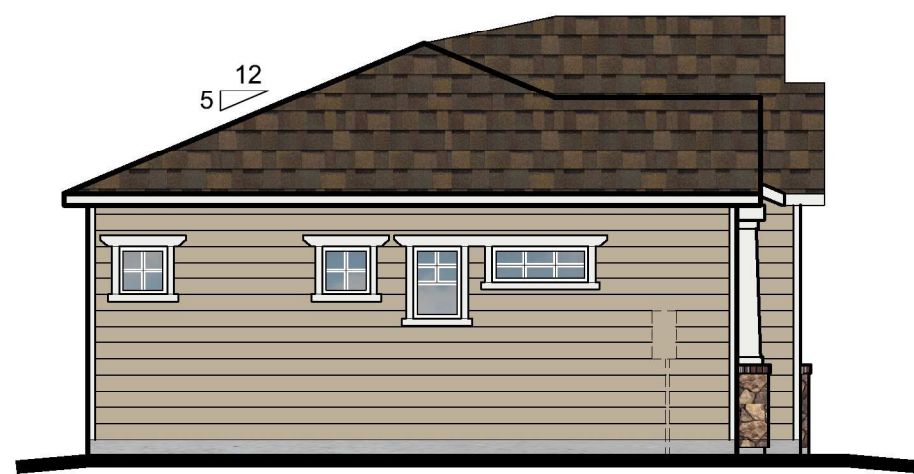
Left Elevation Elevation B 1/8" = 1'-0"
