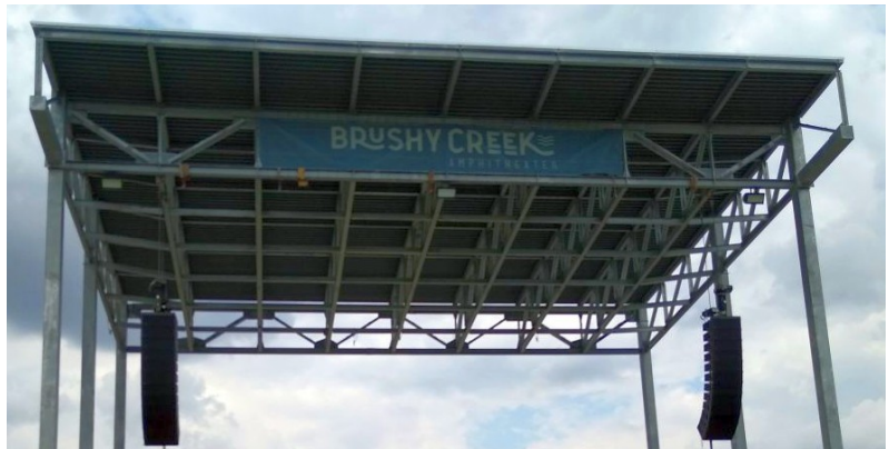
Figure 5.1 Needed speaker hang height and venue roof height. Hanging subwoofers may not be an option unless the hang goes lower.
